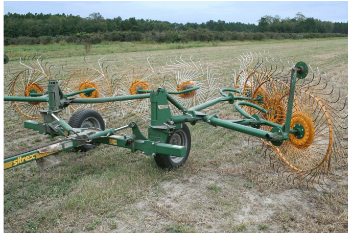
A wheel rake parked at the edge of an alfalfa field in Coffee County, GA after the hay has been harvested.
