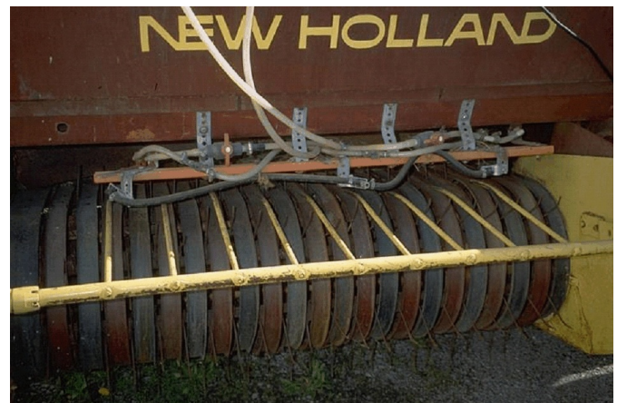
Hay preservatives can cause excessive corrosion on equipment.
